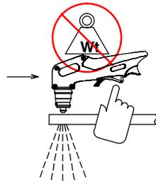
**DO NOT** put pressure on shield when **drag cutting**; instead, slide shield along the surface for proper cutting results.
