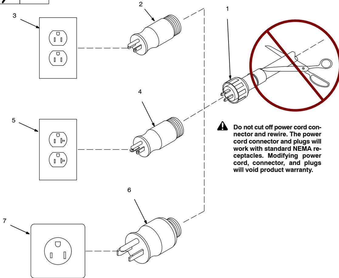
**⚠ Do not cut off power cord connector and rewire. The power cord connector and plugs will work with standard NEMA receptacles. Modifying power cord, connector, and plugs will void product warranty.**
