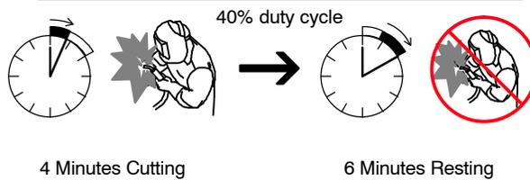
Duty Cycle is percentage of 10 minutes that unit can cut at rated load without overheating.
