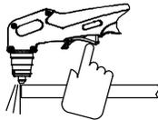
Raise trigger lock and press trigger. Pilot arc starts.
