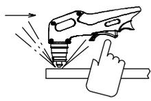
If sparks flare back from surface, this usually is an indication that either travel speed is too fast or amperage is set too low.
