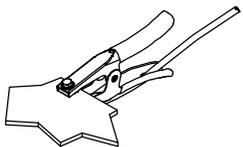
Always connect work clamp to a clean, paint-free location on workpiece, as close to cutting area as possible.
