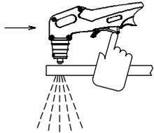
Sparks should pass through the workpiece and out the bottom when cutting.
