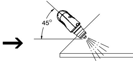
Hold torch at approximately 45° to the workpiece. Raise trigger lock and press trigger. Pilot arc starts.
