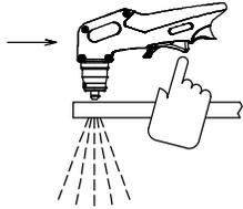
Pulling rather than pushing the torch makes cutting easier. Use a proper guide or template for accurate cutting operations.
