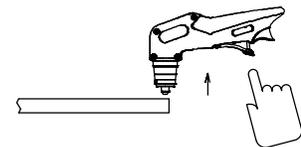
Postflow continues for approx. 20 seconds after releasing trigger; cutting arc can be instantly restarted during postflow by raising trigger lock and pressing trigger.
