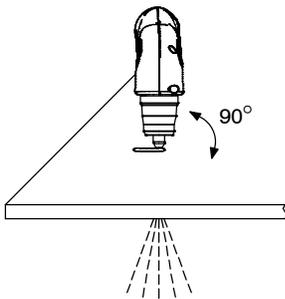
Rotate torch to upright position approximately 90° to surface. When arc has pierced through workpiece, start cutting.
