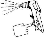
**DO NOT** start pilot arc without cutting as this shortens the service life of the nozzle and electrode.
