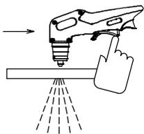
Adjust torch speed so sparks go thru metal and out bottom of cut.
