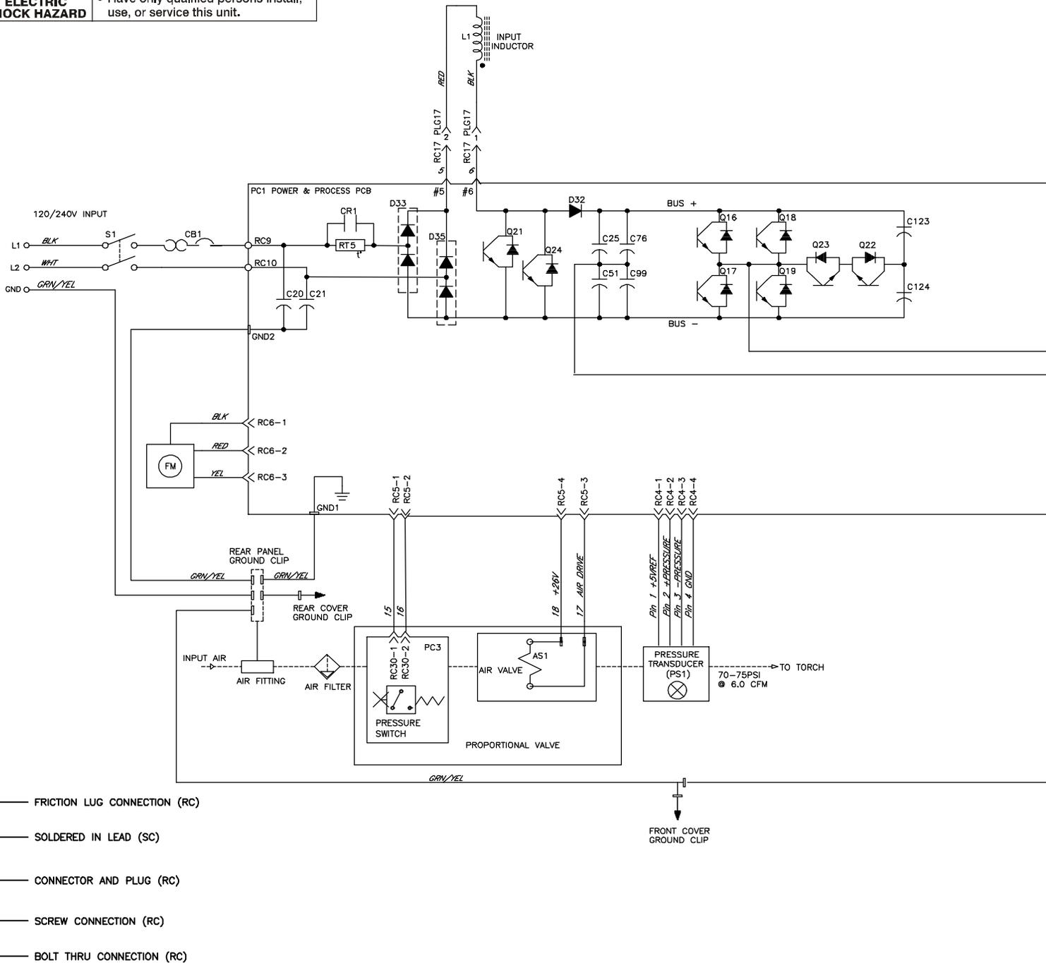
Figure 8-1. Circuit Diagram For AirForce 27i
