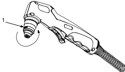
**⚠** Power must be reset whenever the cup shutdown system is activated. **Always turn Off power when changing or checking consumables. Do NOT over tighten torch shield cup. Gently finger tighten cup onto torch.**
