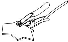
Connect work clamp to a clean, paint-free location on workpiece, as close to cutting area as possible.
