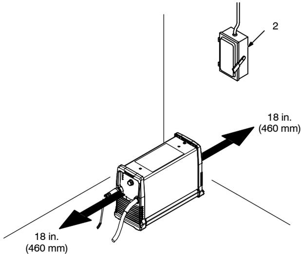
**⚠** Special installation may be required where gasoline or volatile liquids are present – see NEC Article 511 or CEC Section 20.
