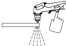
Pause briefly at end of cut before releasing trigger.
