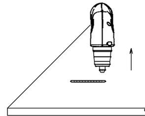
Release trigger. Postflow continues for approx. 20 seconds after releasing trigger; arc can be instantly restarted during postflow by raising trigger lock and pressing trigger.
