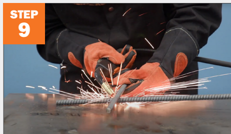
Center 10" piece of rebar near the bottom of the stand and tack weld.
