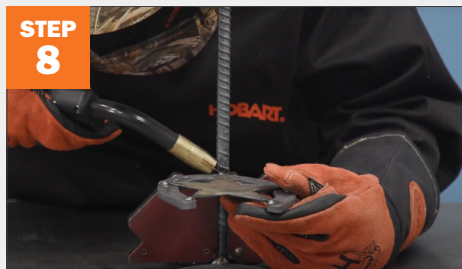
Tack and weld the bottom horseshoes of cup holder to the rebar.
