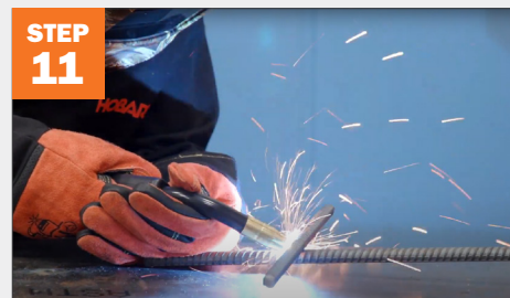
Weld the 10" piece of rebar to create a ground stopper.
