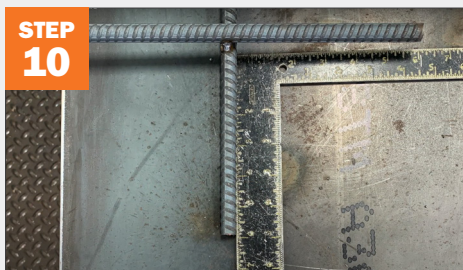
Use the carpenter square, and make sure the two rebar pieces are square.
