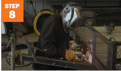
Weld angle iron supports.
