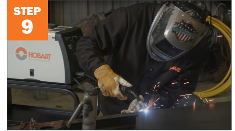
Weld 1/8" steel plate.
