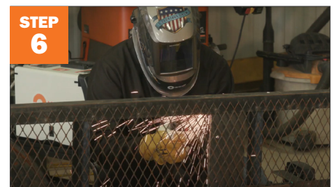
Weld spare tire mounting plate.
