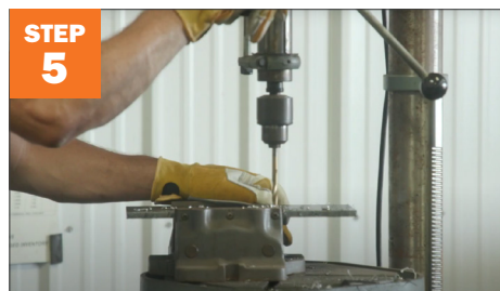
Drill holes for mounting bolts.
