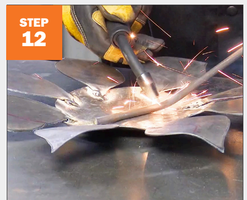
STEP 12 Tack weld stem to the back of the sunflower at different points of contact.
