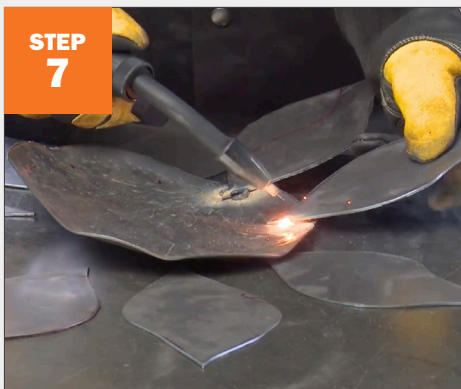
STEP 7 Tack and weld petals to the center circle.
