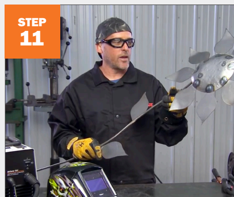
STEP 11 Tack additional petals to the stem at whatever location you desire.
