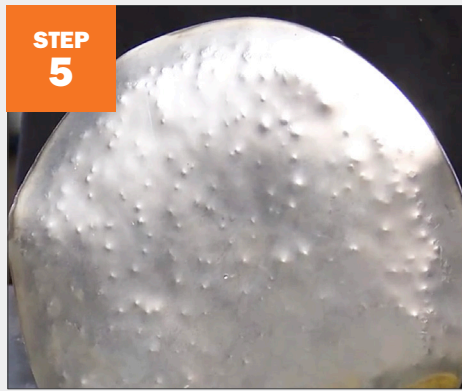
STEP 5 Use a hammer to shape and add texture to the round piece.
