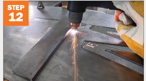
Cut out the inside of each letter, using a scrap piece of metal for a straight edge.
