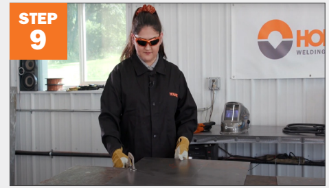
Move material to hang off table, so you are not cutting on the table, secure with a clamp.
