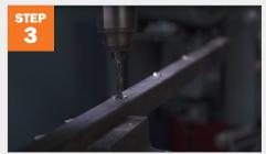
Pre-drill holes in square tubing of where you would like each hook to be placed.
