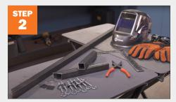
Cut the tubing at 45-degrees on both ends of the long piece and at one end of each short pieces.
