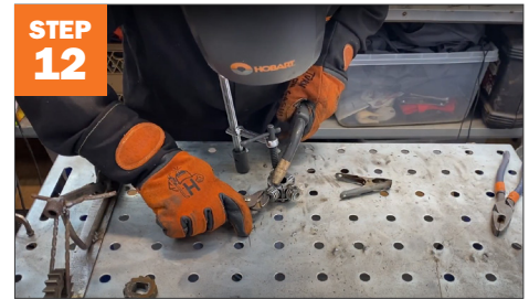
Weld the stack of washers to the engine.
