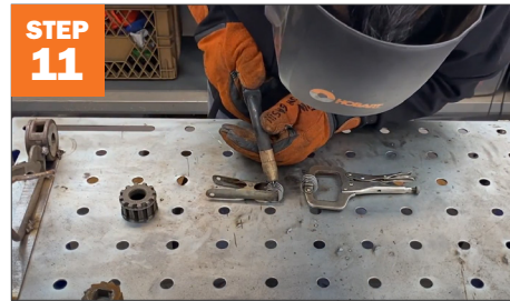
Alternate small and large washers to create cylinders, weld together.
