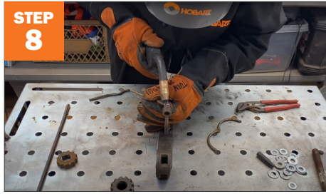
Tack weld the handles to the top of the frame.
