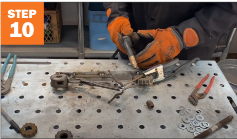
Weld the forks to the front wheel and frame.
