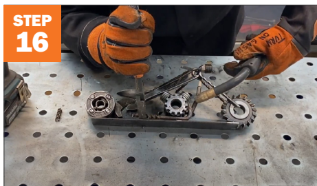
Tack weld exhaust to engine.
