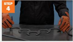
Flip over the welded horseshoes, place two horseshoes at 90-degree angle, and use the carpenter square to make sure the horseshoes are square.
