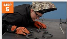
Put rebar in place for the stem, place a horseshoe underneath the rebar to keep it level.
