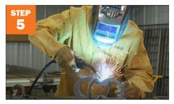
Position the next horseshoes at a 45-degree angle and then weld together, repeat 4 times.
