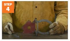
Position the next horseshoe at a 90-degree angle and then weld together, repeat 1 time.
