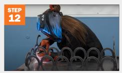
Complete the weld on each side, for extra support weld underneath.
