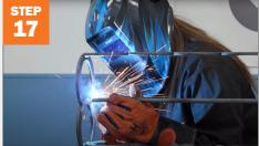
Repeat with the second piece of rebar at the bottom of the top horseshoe, on the same side with the horseshoe opening facing towards you.
