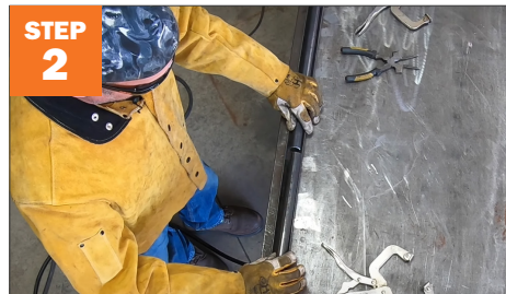
Use angle iron to hold materials straight for welding, if you need to weld two pieces of tubing together.
