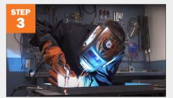
Weld all four corners of the top and bottom sections.
