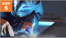
Weld the cross-beam support on both top and bottom square.
