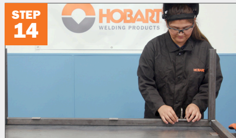
STEP 14 Place and clamp tabs evenly around the bottom of the table frame.
