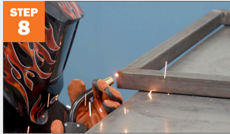
STEP 8 Repeat steps 3-5 to weld two corner frames together. Tip: To prevent burn through, make sure tack weld stops glowing orange before making next tack.
