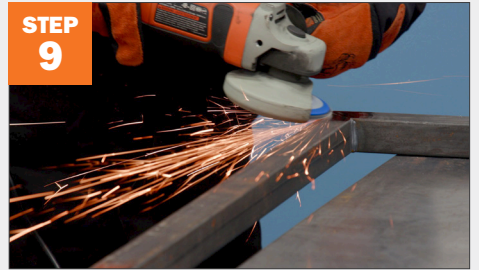
STEP 9 Using a flap disc, grind all the welds flush on each corner.
