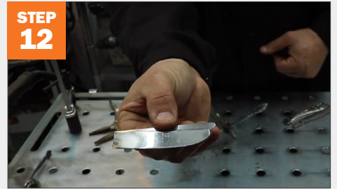
STEP 12 Cut the knife ends to make tips of wings and weld knife tips together.
