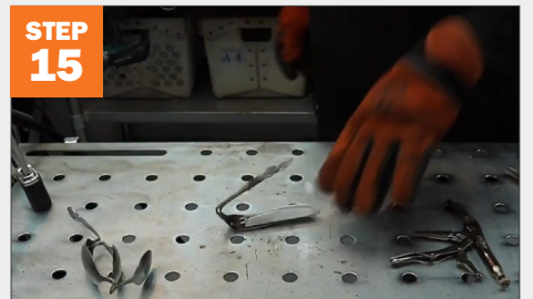
STEP 15 Bend the wing to fit the body.
