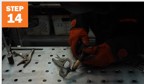
STEP 14 Clamp the wing tips to the forks, and weld the forks to the knives.
