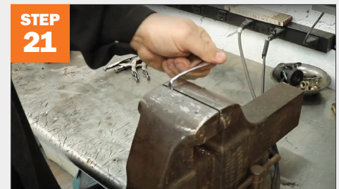
STEP 21 Flatten the spoon to create a perch.
