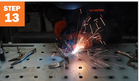
STEP 13 Weld the forks together.
