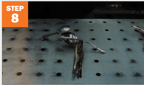
STEP 8 Clamp the back piece to body and weld the back to body.
