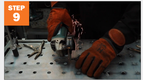
STEP 9 Remove the excess beak material.
