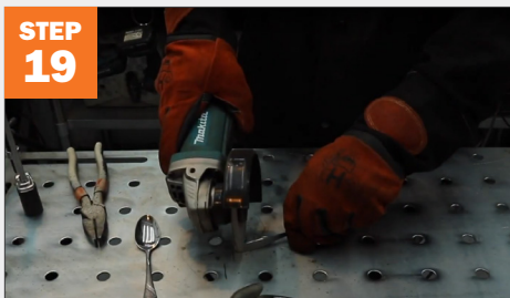
STEP 19 Cut off the excess fork off.
