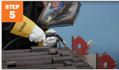
Tack weld each corner.
