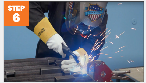
Tack weld all of the middle pieces.
