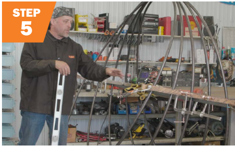
Place and stabilize final two chair rings, and weld.
