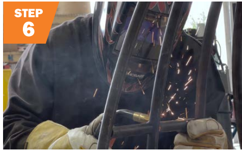
Cut and place two side support bars (2") in between each chair ring, and weld.
