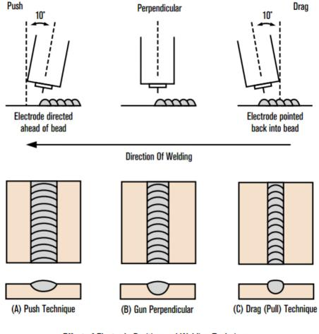
Effect of Electrode Position and Welding Technique
