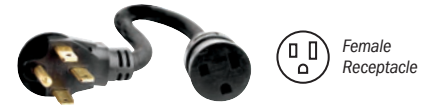
Full KVA Adapter Cord 300517 NEMA 14-50P to NEMA 6-50R. Adapts engine drive 120/240-volt plug to common AirForce 240-volt plug.
