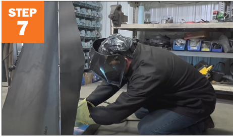
Tack weld the sides to the bottom.
