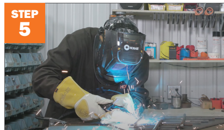
Weld the round bar pieces together.
