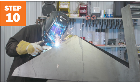
Weld the seams of the sides together.
