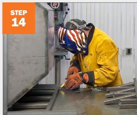
STEP 14 Turn fire pit on its side so it is easier to weld decorative sides in.
