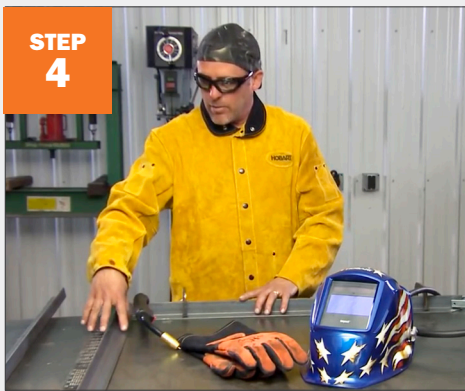
STEP 4 Clamp two corners down to table and make sure it is square.
