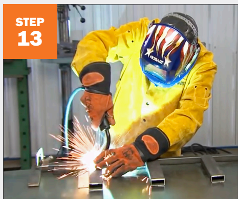
STEP 13 Weld the decorative side pieces. In video: Place 1" x 1" x .065" tubing horizontal on table with three pieces of 1" x 2" x .065" tubing standing on top. Weld together.
