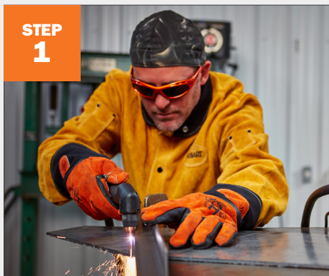
STEP 1 Cut 3/16" plate pieces. Tip: Use a straight scrap piece of metal to help create straight line.
