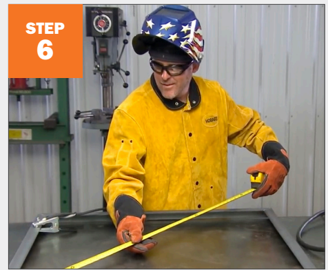
STEP 6 When all four corners are tack welded, flip over and make sure you are squared.
