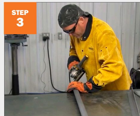
STEP 3 Use a grinder to bevel edges
