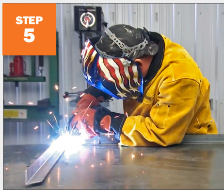
STEP 5 Tack weld corners into place.
