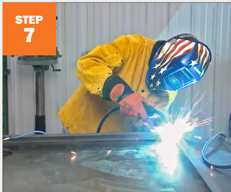
STEP 7 Weld the top of each corner.
